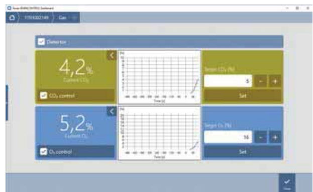
Figure 12: You have full control of the environmental conditions during a run, including the temperature and the \text{CO}_2 and \text{O}_2 levels inside the reader.
