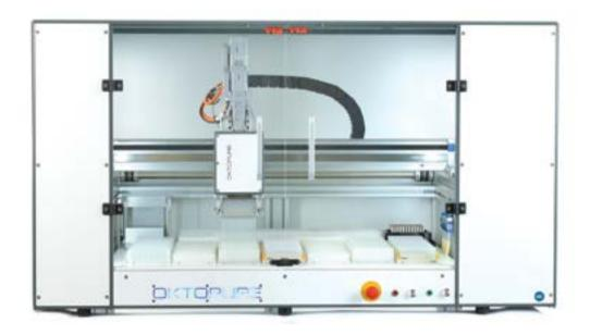
Plant breeders are utilising the rapid and continued advancement of molecular biology-based technologies to dramatically accelerate their breeding programs. The oKtopure platform has been developed to deliver automated DNA extraction from 8 x 96-well microtitre plates in parallel, utilising the proprietary sbeadex magnetic bead-based chemistry.
